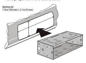
2 When the mounting sleeve is in the correct position, bend several mounting *claws* outward to achieve a tight fit and lock the mounting sleeve into place.
